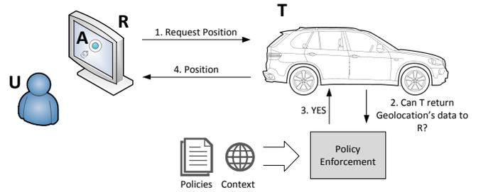
Fig. 3. Example of a request to access a remote device's features. Application A launched by user U in set-top box R requires access to geolocation data provided by car T.
