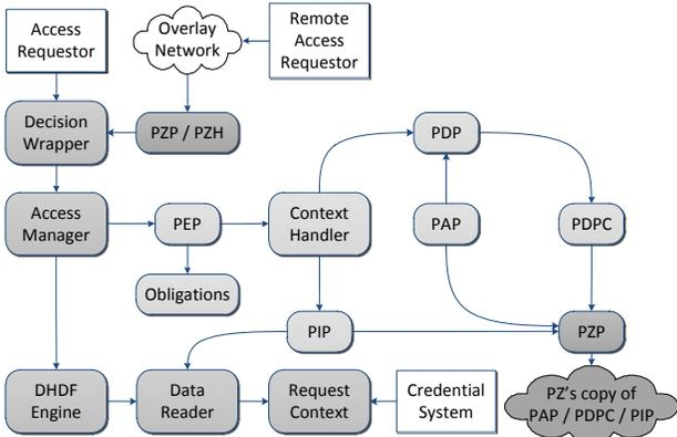
Fig. 2. Components of the *webinos* policy framework on a device. Requests come from either local or remote sources, and are then managed by the Decision Wrapper. Policies are held on a PZP and may depend on data fetched from the rest of the personal zone
